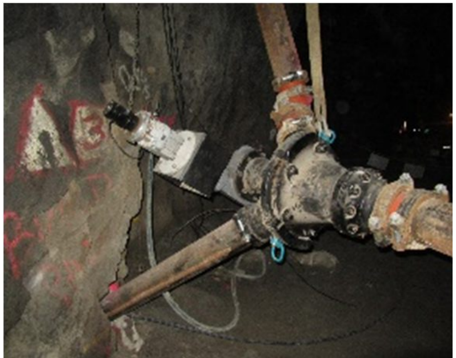
Designed for either manual operation or remote actuation, the automated diverter valve enables mines to quickly and easily divert paste and dump backfill in the event of a blockage. (Photo courtesy of Victaulic)
